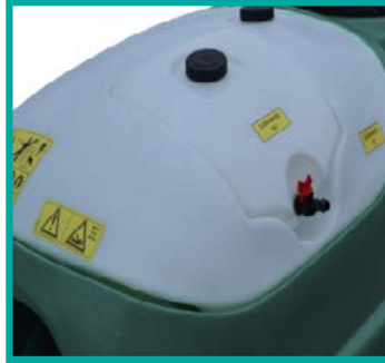
Serbatoio lavamani Hand washing tank
